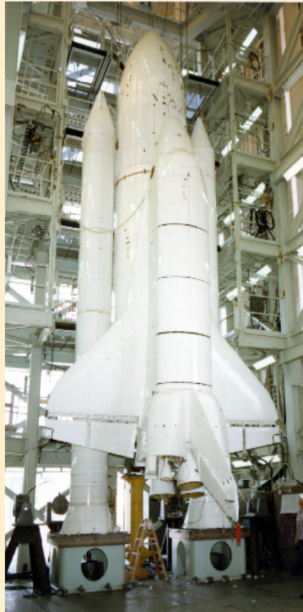
Quarter-Scale Shuttle Test Article positioned in the vibration test fixture, Downey Bldg 288
